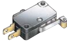
Type 1 / M1 (2) SPDT Mechanical 15 amp @ 125 VAC, ½ amp @ 125 VDC Minimum 50 mA
