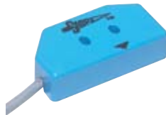
Type E / P1 Sabre Switch (2) SPDT Proximity 1 amp @ 120 VAC, 1 amp @ 24 VDC, 25 Watt Max. Minimum 1 mA
